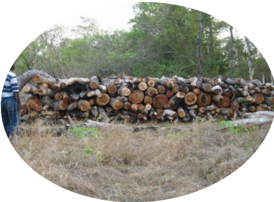
Traditional charcoal production kiln pack up. The way the wood is packed gives big losses during burning, producing less charcoal than it could be possible.
