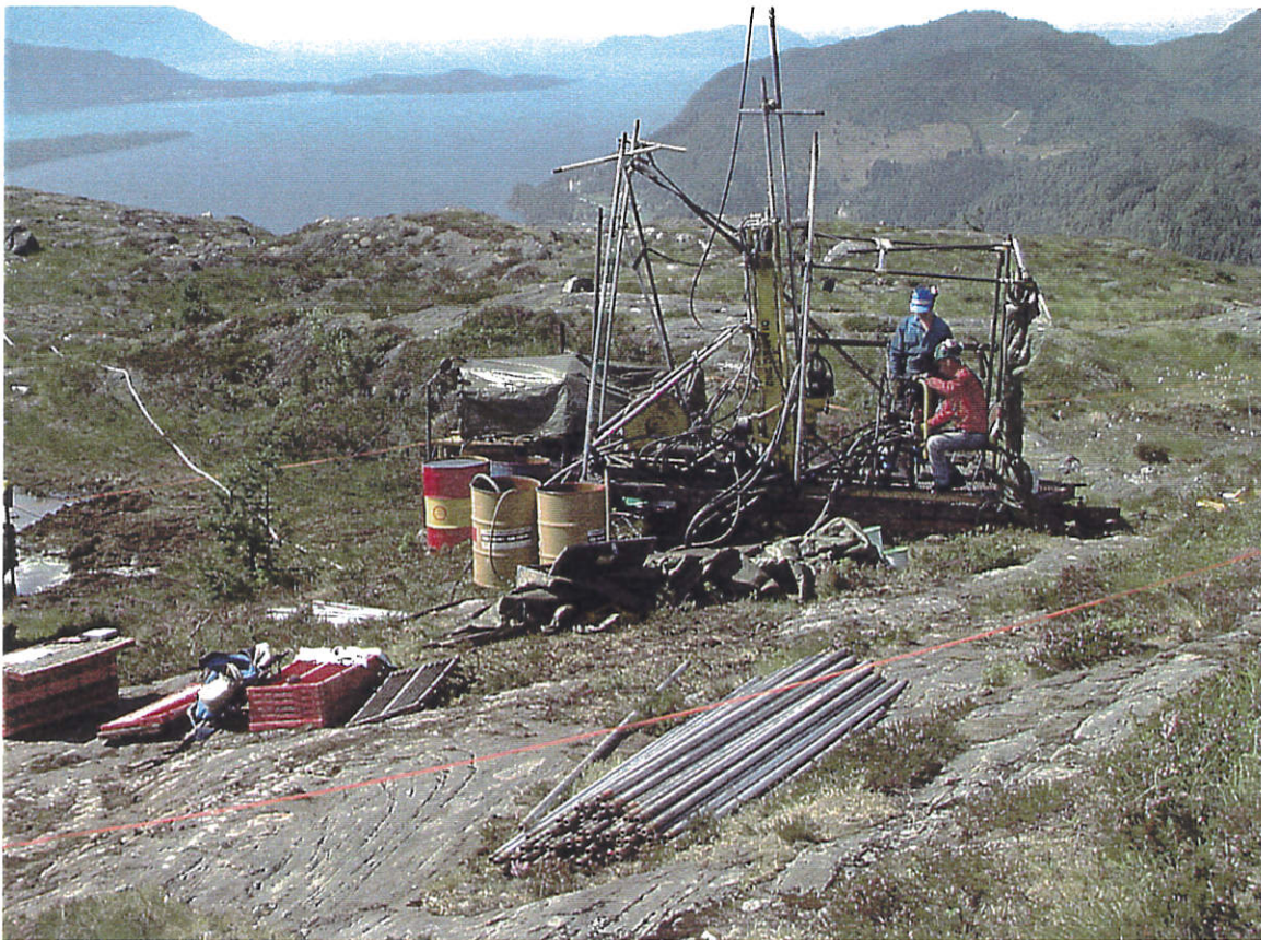
Fig. 10. Exploration drilling at Engebøfjellet
