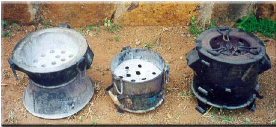
Types of Charcoal Stoves used in Kenya: Center is the traditional non-energy saving. (Source; AFREPREN)
